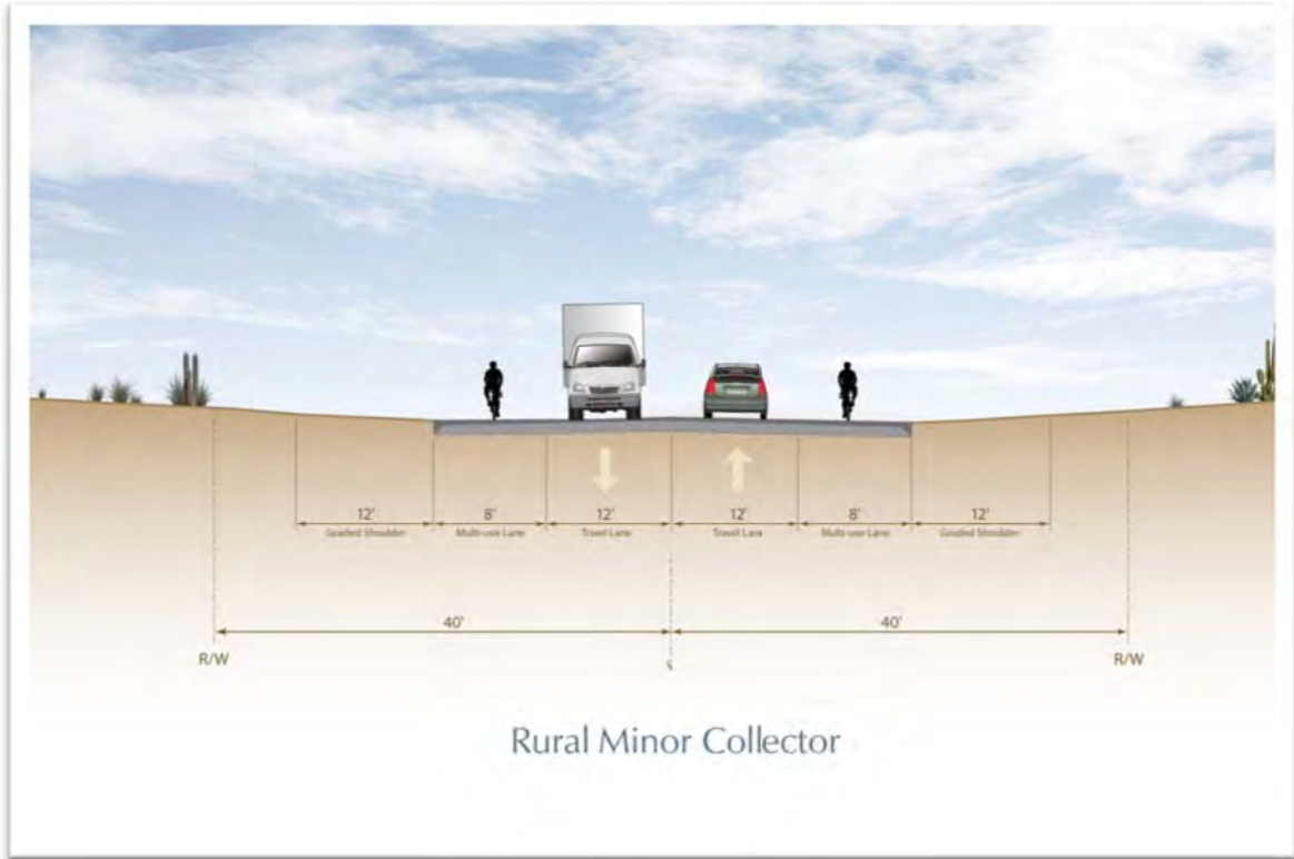
Figure 5 – Rural Minor Collector Cross-Section
