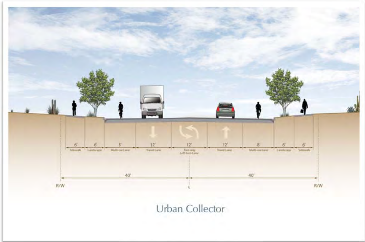
Figure 7 – Urban Collector Cross-Section
