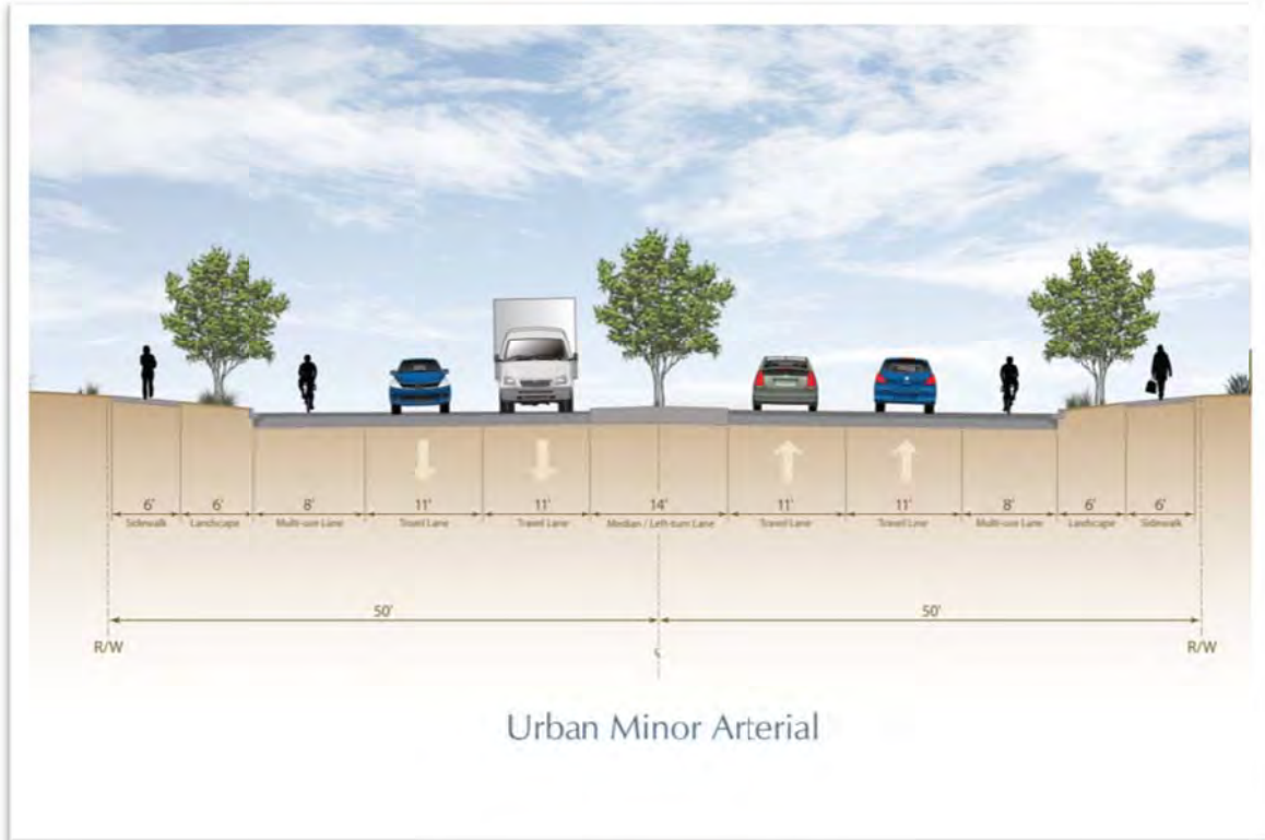
Figure 9 – Urban Minor Arterial Cross-Section
