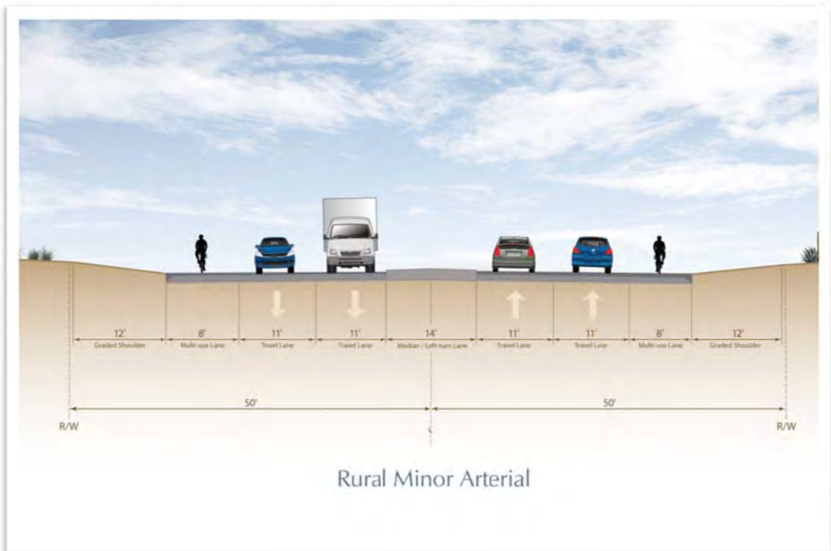
Figure 8 – Rural Minor Arterial Cross-Section
