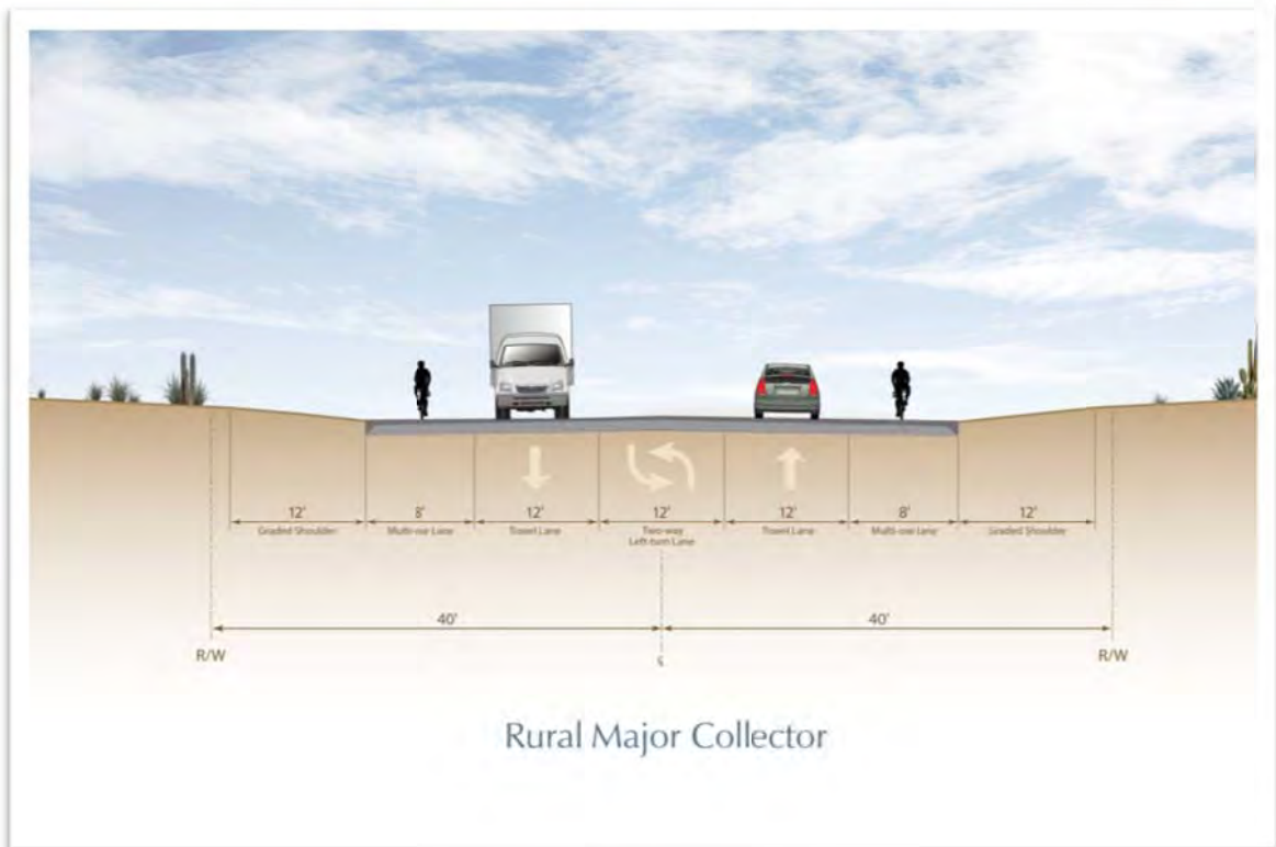
Figure 6 – Rural Major Collector Cross-Section
